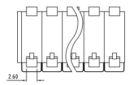
NOTE: Mates with a  $\phi$ 1.1mm pin Part Number Configuration.
